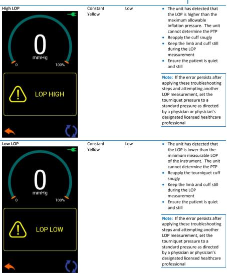
\*In the 'safe state' mode, the pneumatic valve is opened to deflate the cuff. Refer to Alarm Conditions under Section 2 Operating Instructions for more information.
